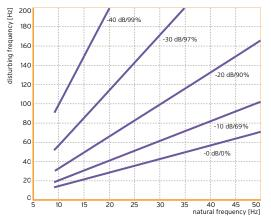
reduction of the transmitted mechanical vibrations by implementation of an elastic bearing consisting of Sylodyn® NF parameter: factor of transmission in dB, isolation rate in %
