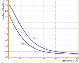
DMA-test (Dynamic Mechanical Analysis); tests within linear area of the load deflection curve, at low specific loads
